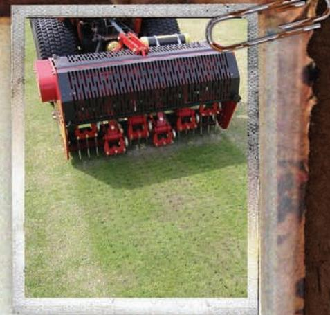
The Verti-Drain Mustang 7110 is a fast Verti-Drain with a working width of 40" (1.0m), penetrating up to 6" (150 mm) deep. The tines can be adjusted to the vertical position for hollow coring, or to the 'kick' position for solid tine use. It is a simplified Verti-Drain model, containing a one-speed gearbox, and considerably less weight (approx 725 lbs/330kgs) allowing for use of a 13-15 hp tractor. The 7110 is supplied without a rear roller.
